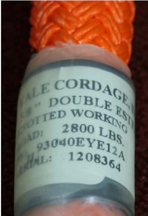
Above rope showing safe working load
