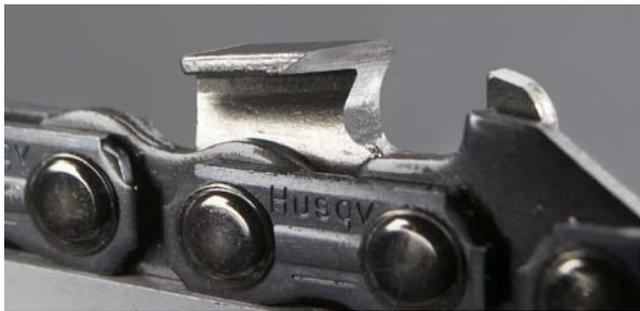
checking the cutters for damage, selecting the first one to sharpen
