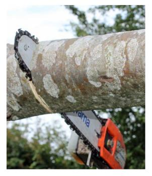
There may be occasions when the powered pole pruner becomes trapped in a cut. It is important to know how to remove it without damage to the pole pruner or the branch being severed.
